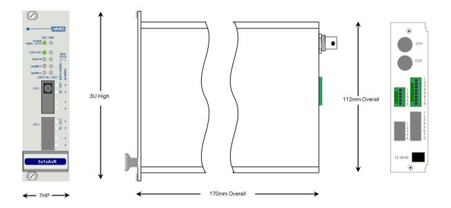
The **AMG5414A9R** is a rackmount receive unit designed to transmit & receive one bi-directional data signal, one bi-directional alarm and one bi-directional audio channel over a single Multimode optical fibre.
